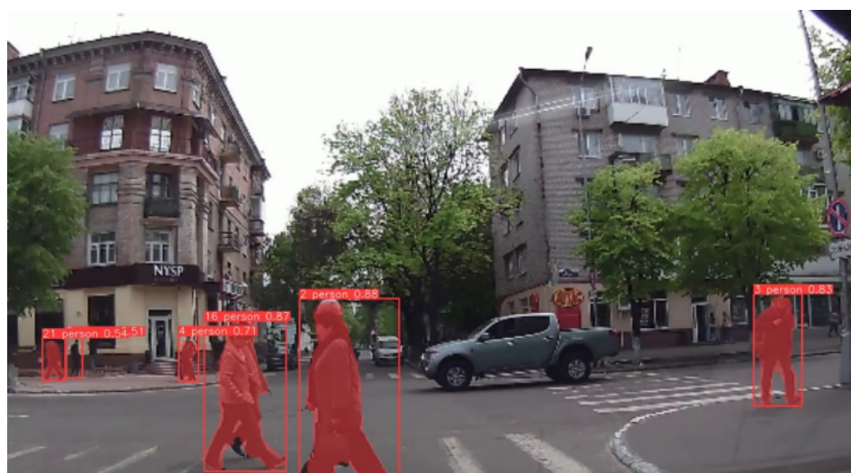
Figure 9. Detection and tracking of pedestrians using YOLOv8n-seg and StrongSORT_P.
