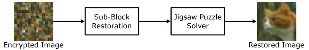
Figure 4. Proposed jigsaw puzzle solver-based attack
