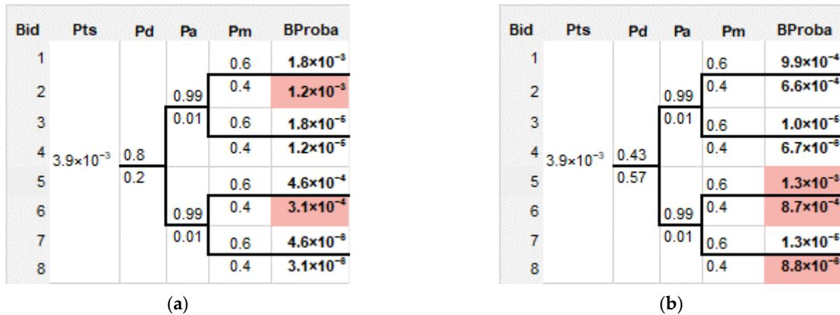
Figure 20. Event trees for the intrusion of an unauthorized drone in LIMC 35 departure path when takeoff is occurring [14]. (a) <1 km from runway. (b) >1 km from runway.
