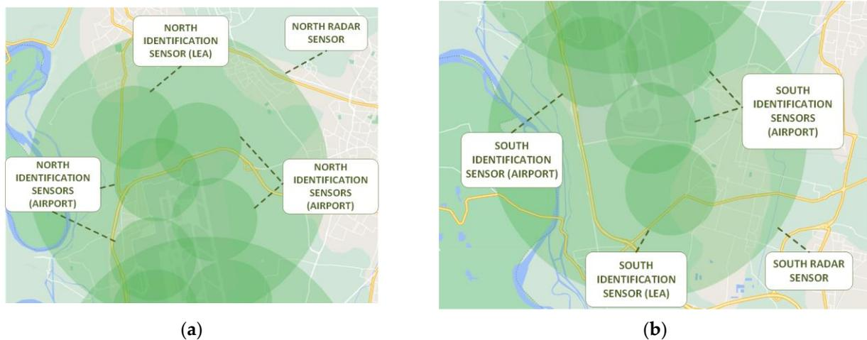
**Figure 12.** Displacement of counter-drone sensors for solution scenarios. (a) North part of LIMC. (b) South part of LIMC.
