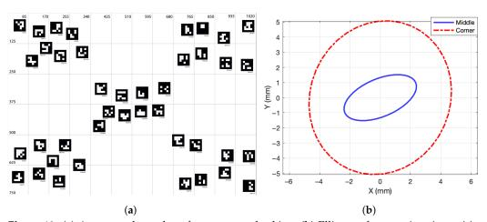
**Figure 10.** (a) Aruco markers plane for accuracy checking; (b) Ellipses of uncertainty in position (95% confidence level with k = 2.4478 [28]).
