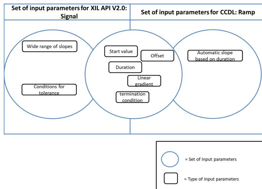
**Figure 4.** The intersection of the input parameters for the ramp function in XIL and CCDL.
