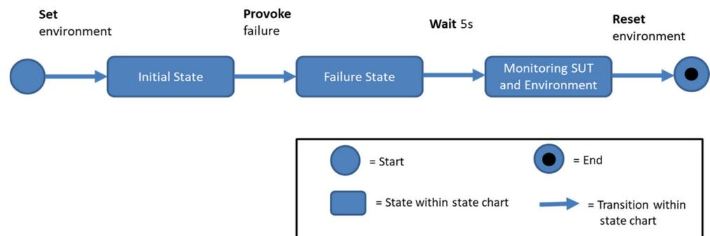
**Figure 1.** Basic steps of a test case.
