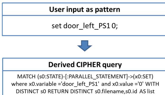
Figure 13. Example for the mapping of a pattern to a CYPHER query.
