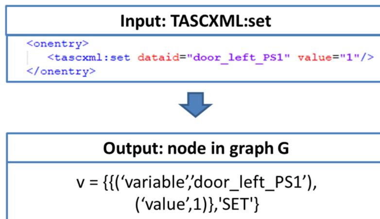
Figure 9. Example for mapping the TASCXML command set to a graph node.
