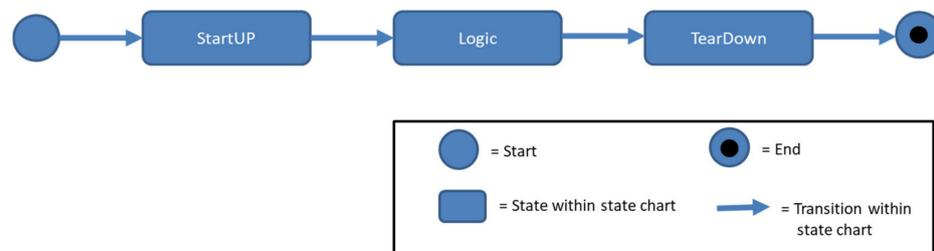
Figure 7. Basic Structure of a test case in SCXML.
