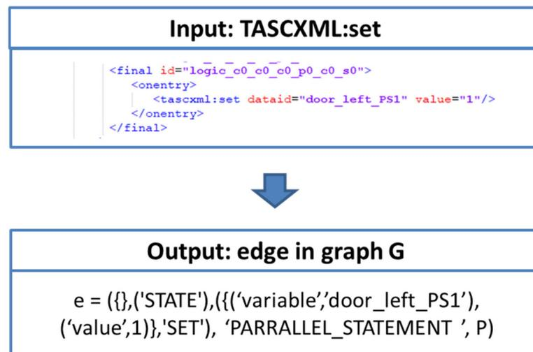
**Figure 10.** Example for mapping the TASCXML: set to a graph edge.
