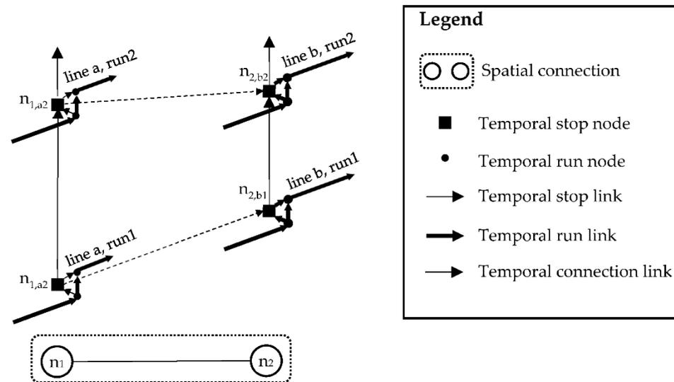
Figure 8. Spatiotemporal connections of an interchange node.
