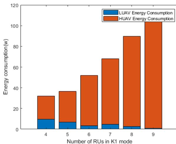
Figure 5. Relationship between the number of RUs selecting K1 mode and the energy consumption proportion of upper and lower unmanned aerial vehicles.
