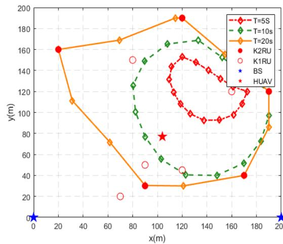
**Figure 2.** Optimized trajectory of the UAV under different flight periods.
