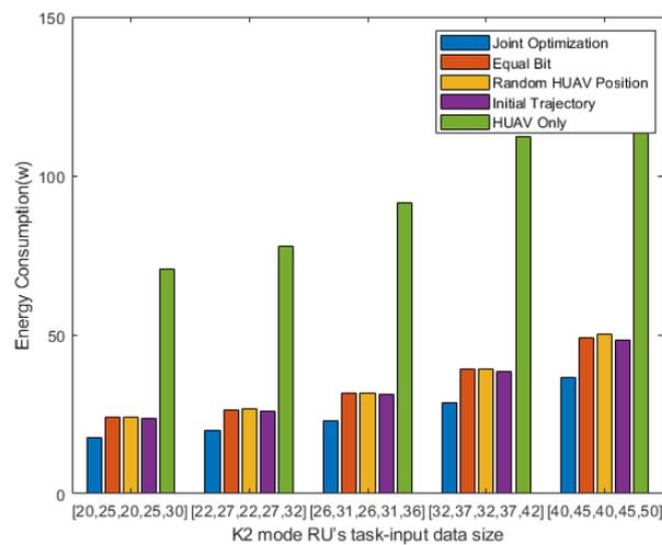
**Figure 3.** The relationship between the RU’s status size and each scheme’s energy consumption in K2 mode when the flight time of the UAV is 20 s.
