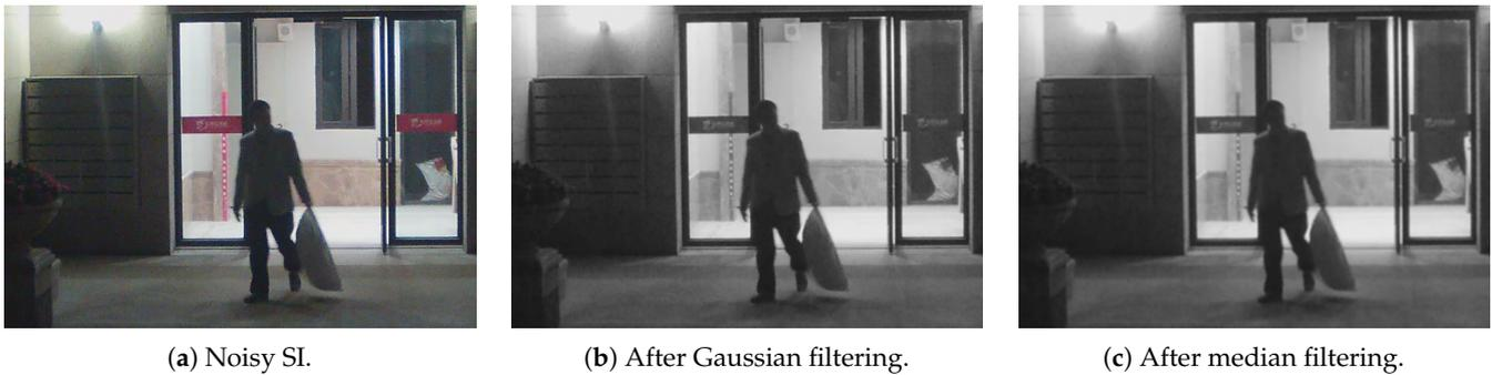
**Figure 3.** Examples of noisy images and denoised gray images. The noise in the low-light and flat regions is reduced after Gaussian and median filtering.
