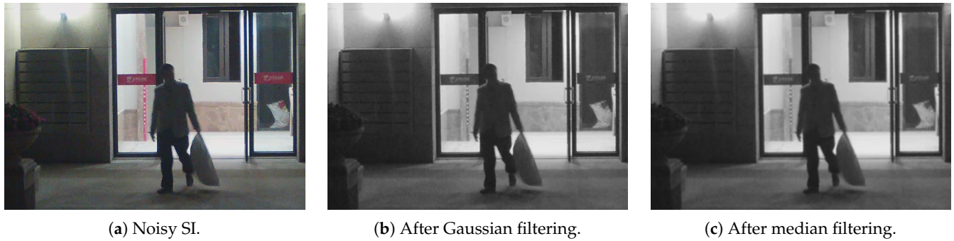
Figure 3. Examples of noisy images and denoised gray images. The noise in the low-light and flat regions is reduced after Gaussian and median filtering.
