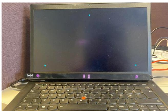
**Figure 6.** Eye-tracker placement and calibration window. Calibration software shows six points in two parts.
