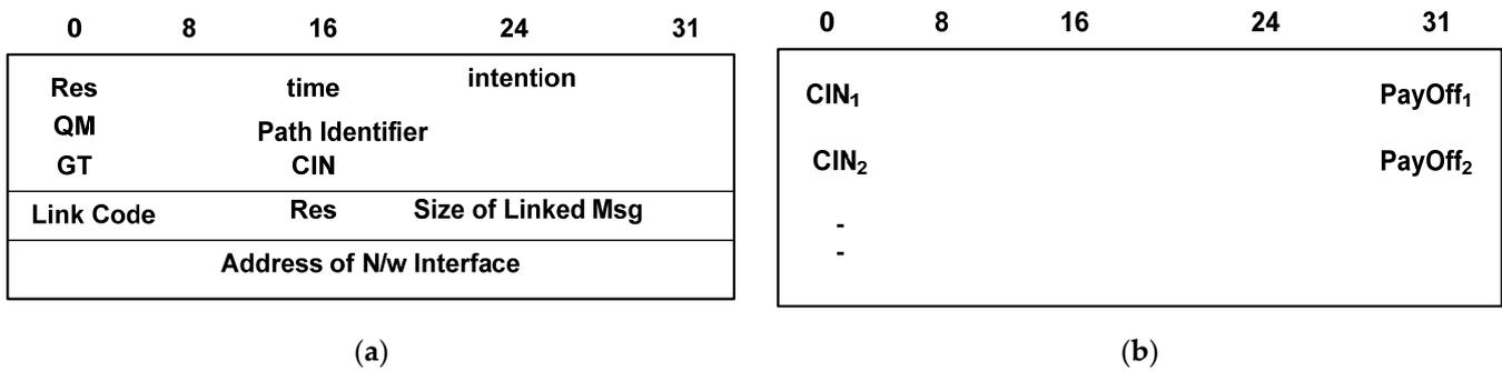
**Figure 2.** Format of newly formulated control message: (a) format for  $C_{msg1}$ ; (b) format for  $C_{msg2}$ .
