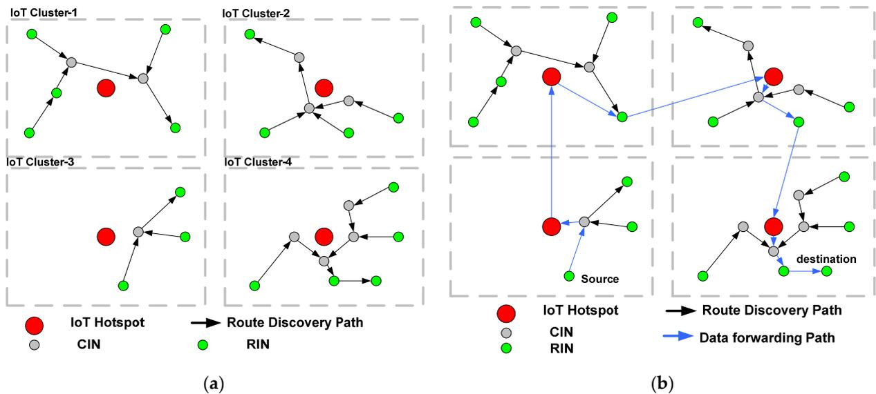
**Figure 5.** Simulation environment of the proposed scheme: (a) IoT cluster formation and routing initiation; (b) Inter-cluster data forwarding.
