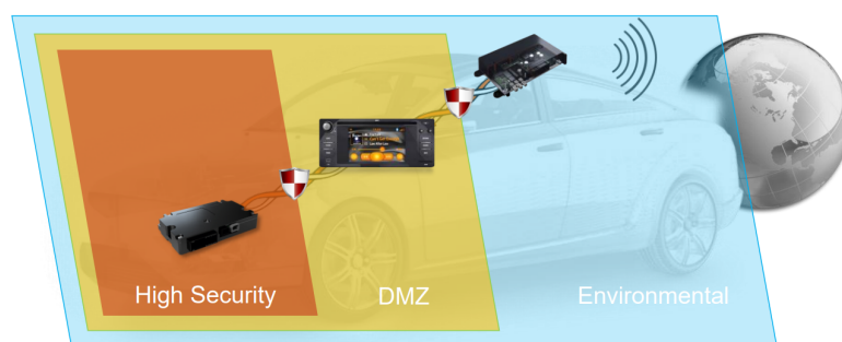
Figure 19. Representation of SEIS Zone Model with Three Zones [13].
