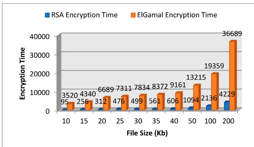
**Figure 9.** Graphical representation of RSA and ElGamal encryption time.
