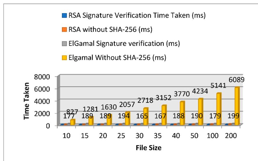
Figure 12. Graphical analysis of the signature verification process of RSA and ElGamal algorithms.
