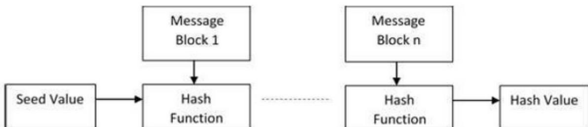
Figure 4. Schematic illustration of hashing algorithms.
