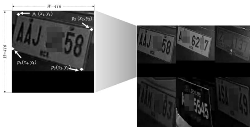
**Figure 1.** Example plate images from data set. Each image contains a single randomly oblique plate with size of  $416 \times 416$ . We manually mark four corners of  $p_i$ ,  $1 \leq i \leq 4$ , for supervised training. The plate numbers are partly blurred for privacy reasons.
