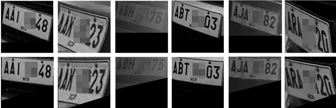
**Figure 4.** Plate images before the transformation (top row) and the corresponding rectified images (bottom row) by using the four-corner predictions from the hybrid model. Parts of the plates are blurred for privacy reasons.
