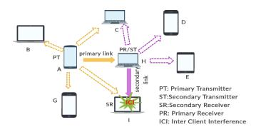
Figure 1. Inter-Client Interference in Ad hoc Networks.
