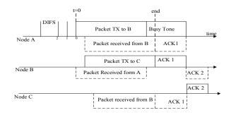
Figure 7. Frame transmission sequence of contraflow [14] in asymmetric link.
