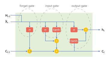
Figure 4. Structure of the repeating LSTM module.
