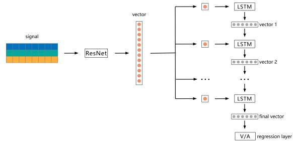
**Figure 6.** ResNet-LSTM model. The signal is first fed into ResNet as a three-channel input (phasic, tonic, and origin).
