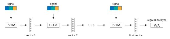
**Figure 5.** The LSTM model. The signal is fed into each LSTM module point by point, and each point contains three channels (phasic, tonic, and origin).
