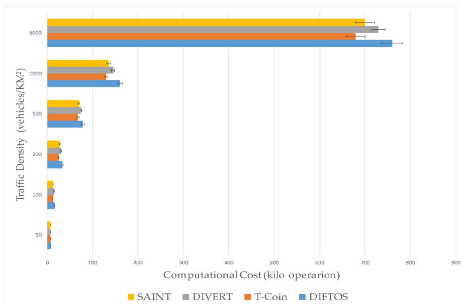
**Figure 11.** Traffic density vs. traffic server computational cost.
