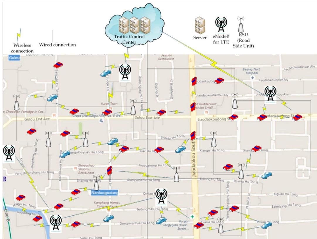
Figure 1. Vehicular navigation architecture.
