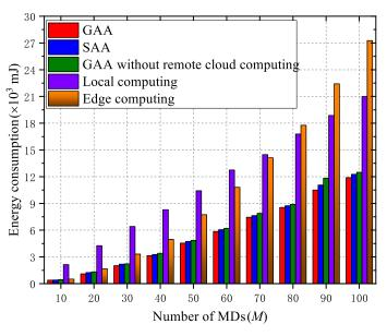
**Figure 4.** Illustration of the calculated minimum consumed energy results by adopting five different computing and offloading schemes, i.e., local computing, edge computing, GAA without remote offloading, and GAA as well as SAA methods.
