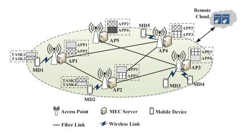
**Figure 1.** A multi-task multi-server MEC architecture: MEC servers deploying at the access points can process various types of tasks simultaneously. MDs can offload the tasks to MECSs or RCC.
