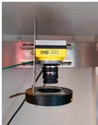
**Figure 7.** Image acquisition platform.
