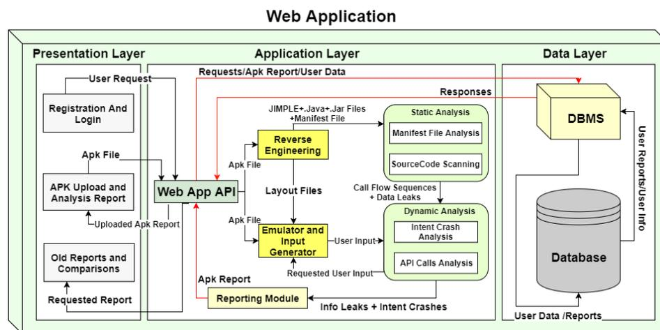
Figure 1. ANDROSHIELD Proposed Architecture.
