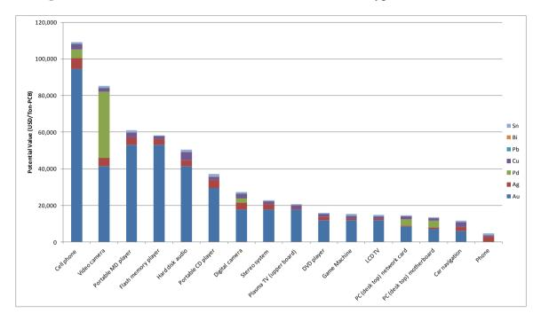
Figure 4. Economic value of metals contained in different types of circuit boards.
