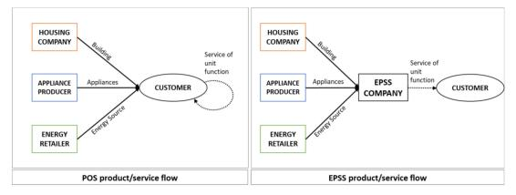
**Figure 1.** Energy, product and service flow in product oriented systems (POS) and energy product service systems (EPSS).
