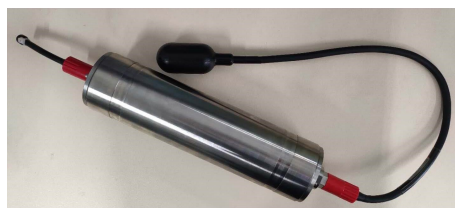
Figure 14. Hydrophone: signal conditioning, low-noise cable and data acquisition.
