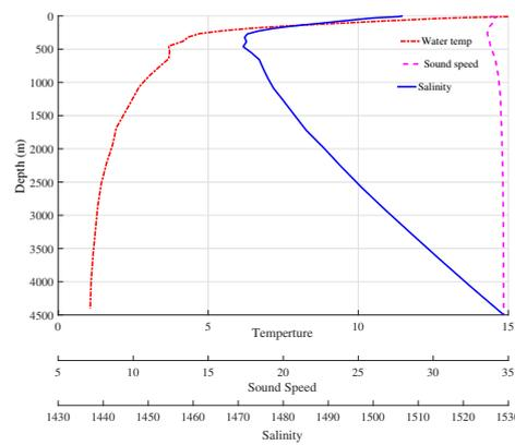
**Figure 7.** Distributions of sound speed profile (blue solid line), temperature (red dash-dotted line) and salinity (pink dashed line) for the depth from the ocean surface to bottom at the position of CTD.
