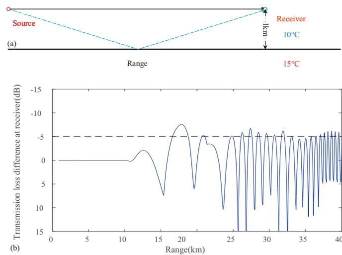
**Figure 2.** (a) A simplified model of front environment source and receiver located 1 km from  $xz$ -plane and (b) frontal reflection effects on the sound pressure field, the curve is the difference transmission loss between a direct wave and a direct plus horizontal reflected wave.
