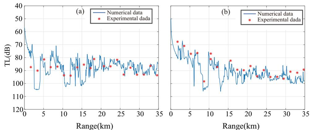
**Figure 18.** Comparison of Transmission Losses between numerical and experimental results for 175 m depth of hydrophone, (a) explosive source at depth 100 m and (b) at 200 m.
