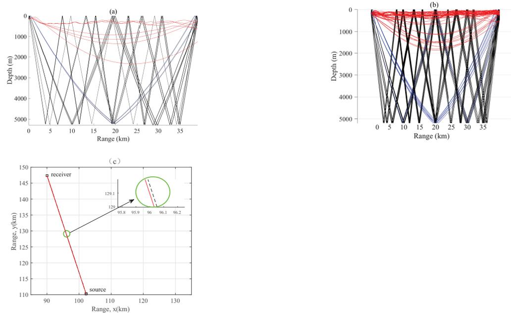
**Figure 21.** Comparison of sound rays between in (a) 2-D and (b) 3-D environment. Subfigure (c) is the top view of sound rays in 3-D simulation which showed horizontal refraction phenomenon. In the picture, red solid line is the acoustic ray and black dotted line is direction from source to the receiver.
