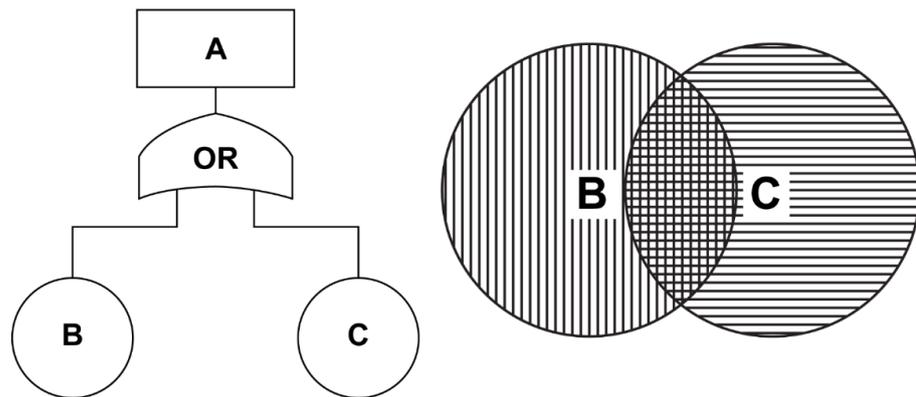
**Figure 3.** Logic of OR gate for fault tree analysis (FTA).
