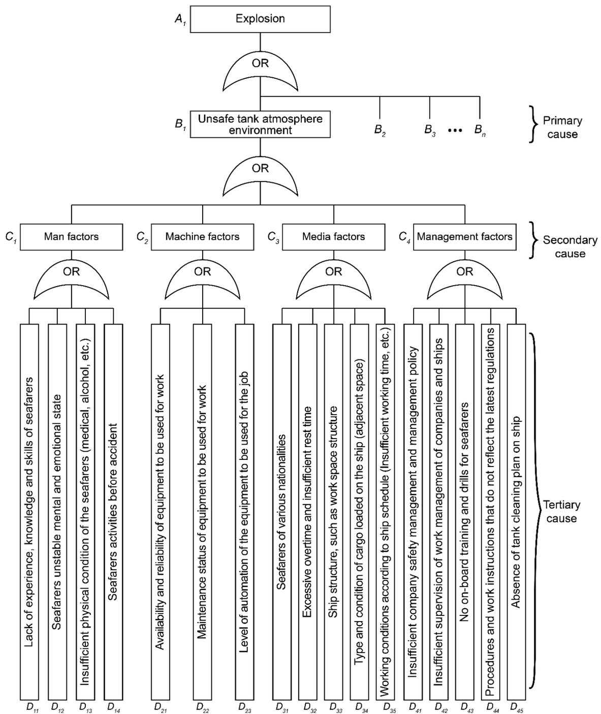
Figure 2. Fault tree diagram for analysis of explosion accidents caused by unsafe tank atmosphere environment.
