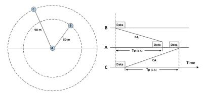
**Figure 1.** An example of two sender nodes (*B* and *C*) simultaneously send packets to node *A* in the same time slot and their transmitted packets arrive at node *A* with no collision due to the distance differences of sender-receiver pairs.
