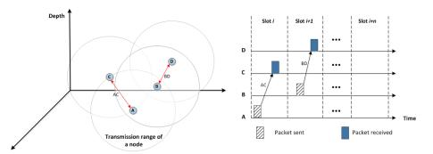
Figure 3. An example of exposed terminal problems.
