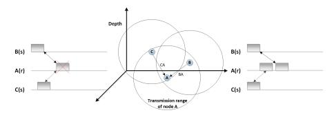
Figure 4. How long propagation delay highly affect the underwater MAC protocol designs.
