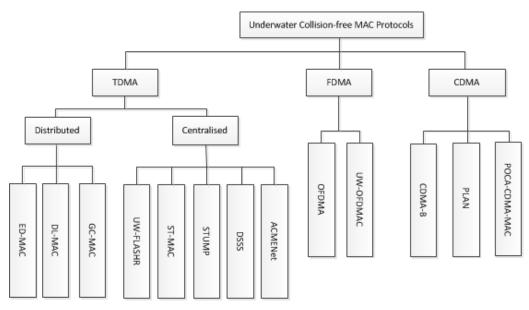
Figure 7. Classification of collision-free medium access control (MAC) protocols for UWSNs.
