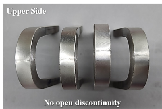
Figure 7. Appearance of the specimen after the bend test.
