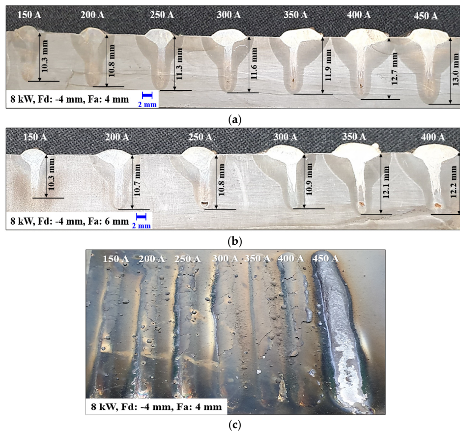
Figure 4. Penetration depth and weld face spatter aspects observed during laser-MIG hybrid welding conditions of high-Mn steel. (a) Macro cross section of the specimen for a power output of 8 kW, F_d = -4 mm, and F_a = 4 mm; (b) macro cross section of the specimen for a power output of 8 kW, F_d = -4 mm, and F_a = 6 mm; (c) weld face spatter aspect after the BOP test.
