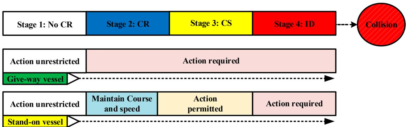
**Figure 1.** Stages and collision-avoidance actions that should be taken by two vessels. The four stages are divided into (1) no risk of collision, (2) risk of collision, (3) close-quarter situation and (4) immediate danger stage, and are displayed in white, blue, yellow and red colors, respectively.
