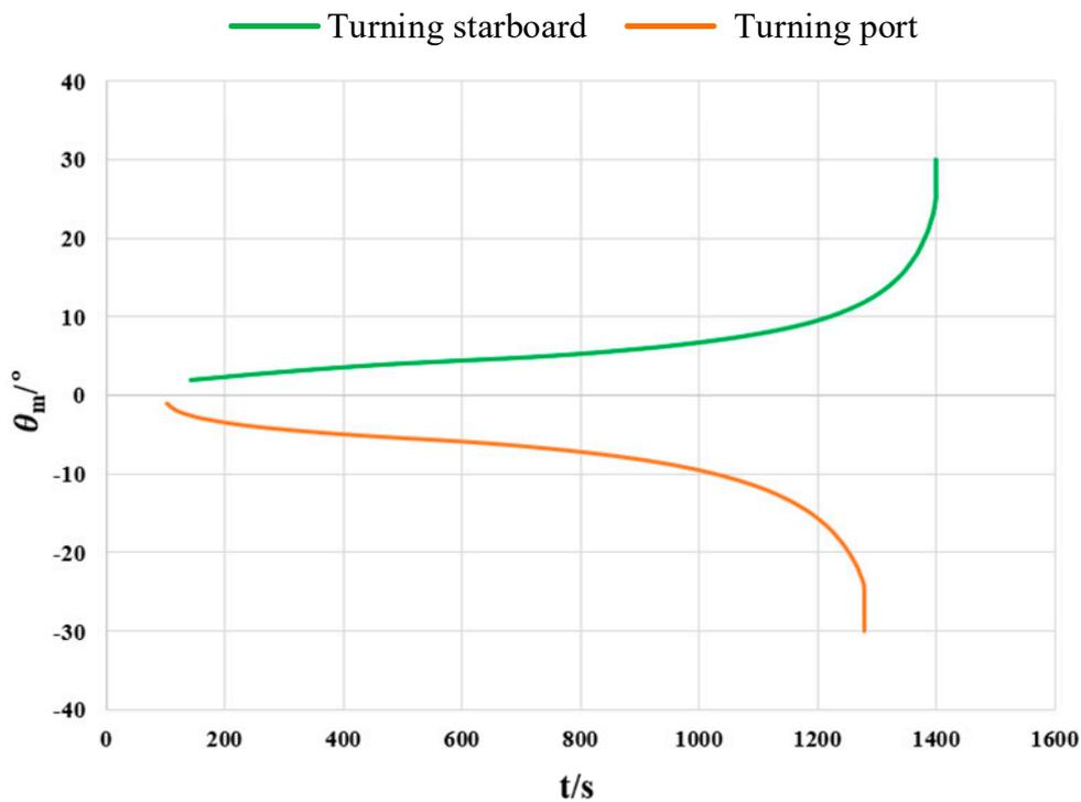
Figure 12. Minimum course alteration angles at different times when the ship domain is not violated.
