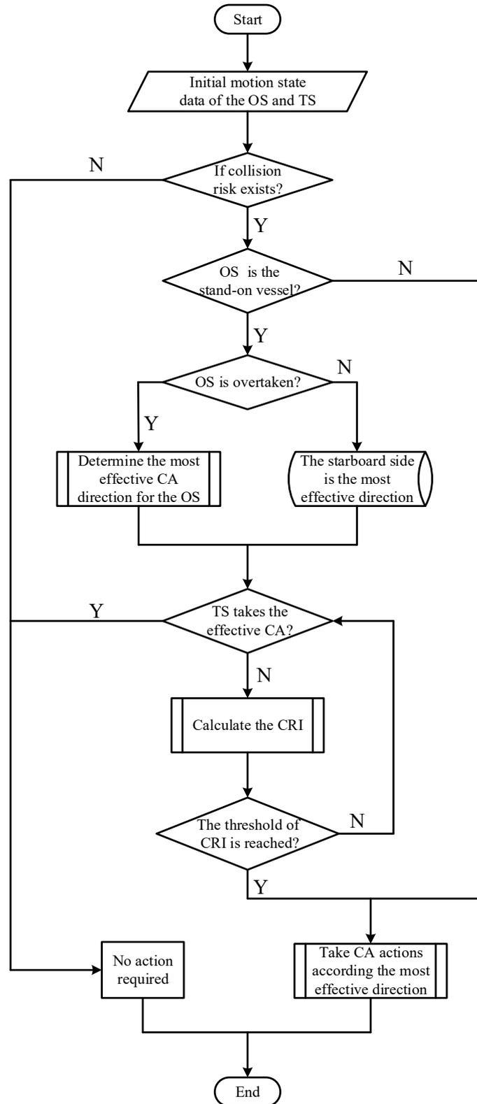
Figure 9. Flowchart of the ACA decision-making method for the stand-on vessel.
