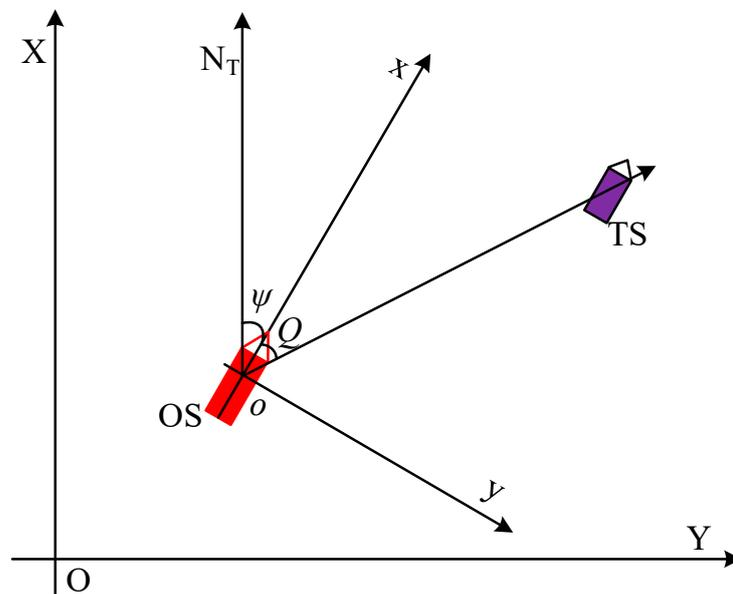
**Figure 2.** Two-coordinate systems.  $XOY$  is the fixed coordinate system and  $xoy$  is the ship coordinate system.  $\psi$  and  $Q$  represent the true course of the OS and relative bearing from the TS.
