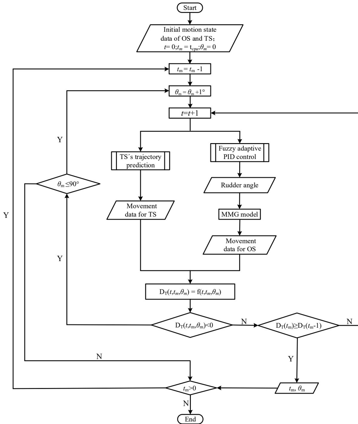
Figure 7. Numerical method of the minimum course-alteration angle based on time.
