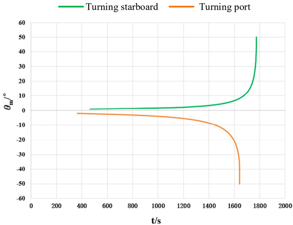
Figure 13. Minimum course alteration angle under different times when the collision domain is not violated.
