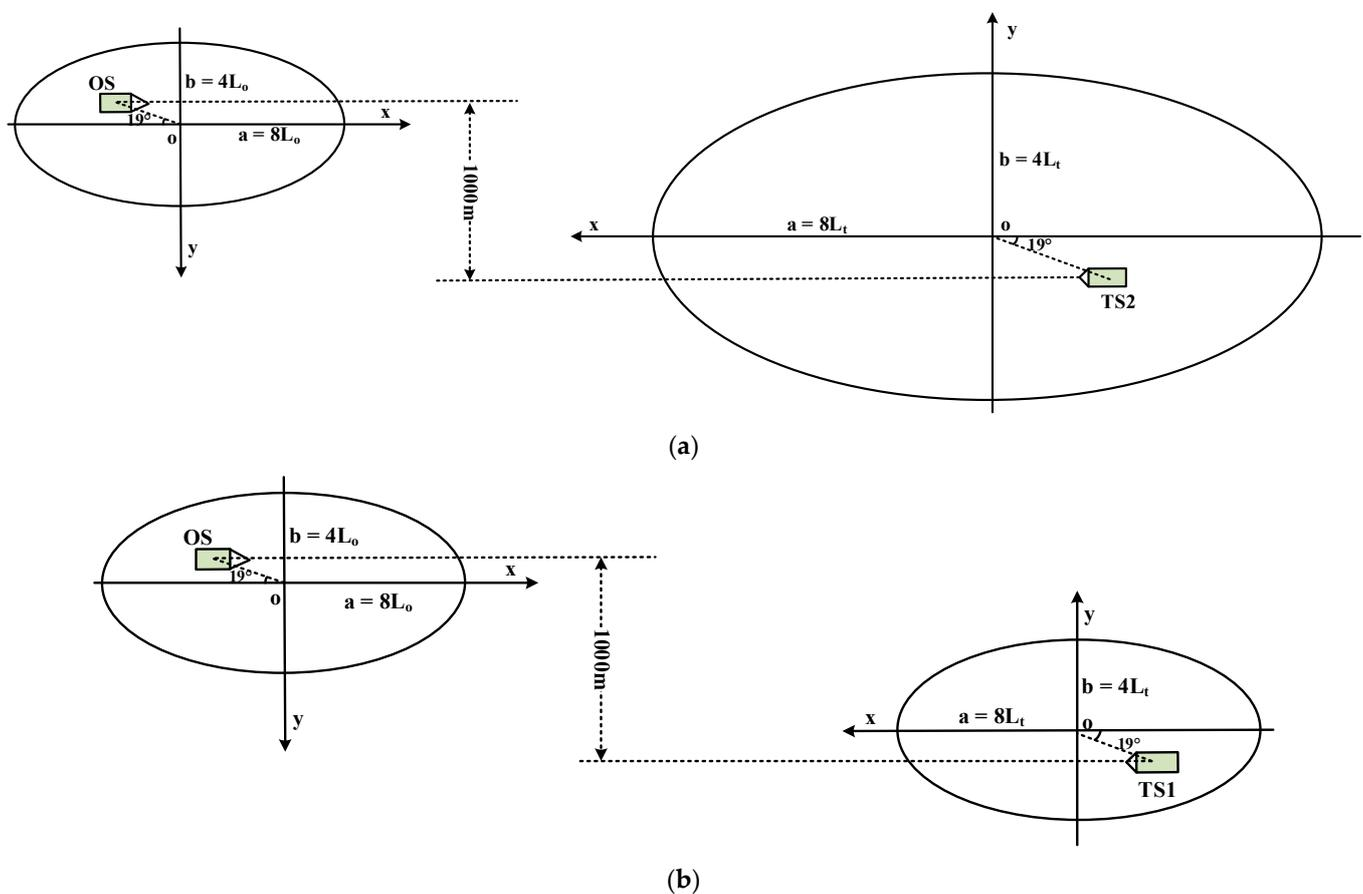
**Figure 3.** Two different encounters in a head-on situation. The lengths of  $L_o$ ,  $L_{t1}$  and  $L_{t2}$  are 160, 336 and 160 m, respectively. (a,b) are variables that can be set accordingly based on the captain’s experience and the ship’s speed. The radius  $a$  and  $b$  of the elliptical ship domain in this experiment are set to 8 times and 4 times of its own LOA, respectively.
