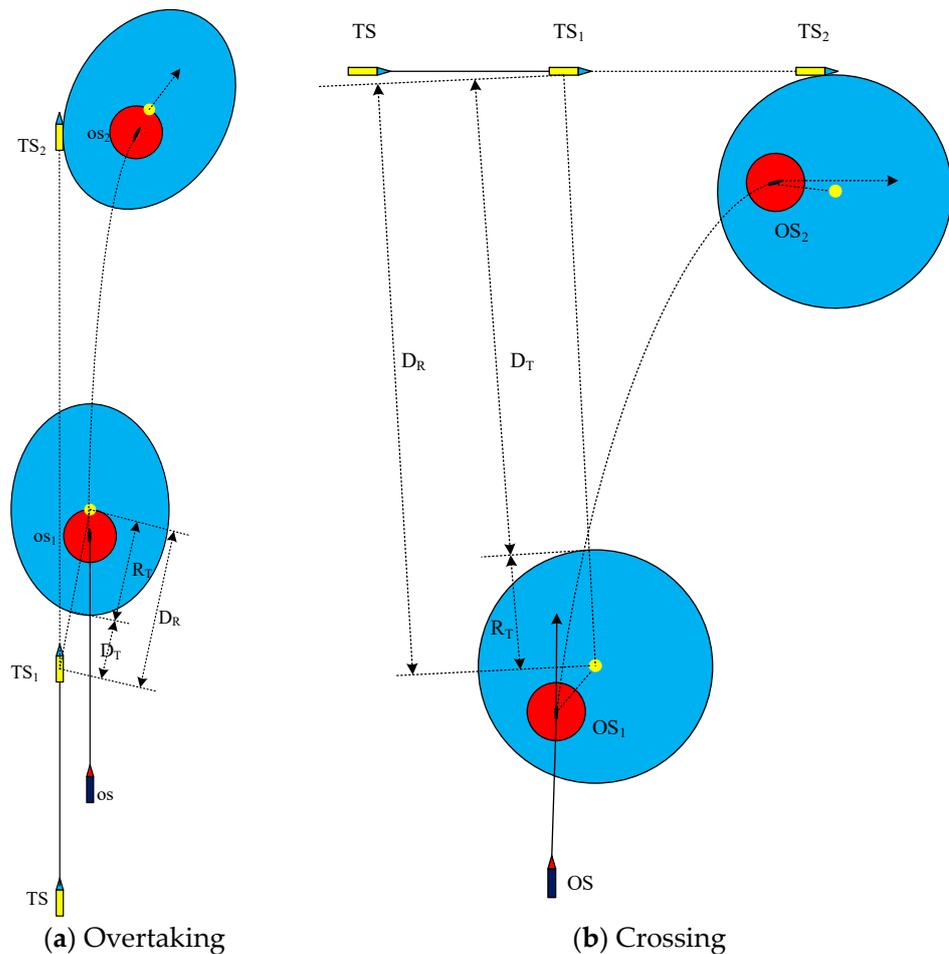
**Figure 6.** Collision-avoidance action by the stand-on vessel in an overtaking/crossing situation.
