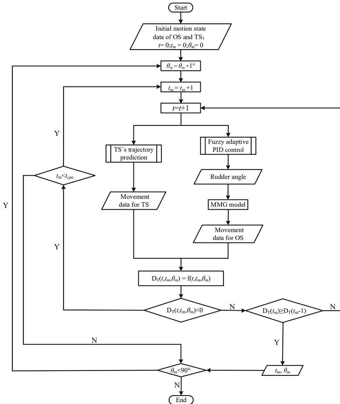
Figure 8. Numerical method of the latest steering time based on the course-alteration angle.
