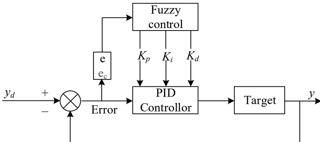
Figure 5. Principle of fuzzy adaptive PID control.
