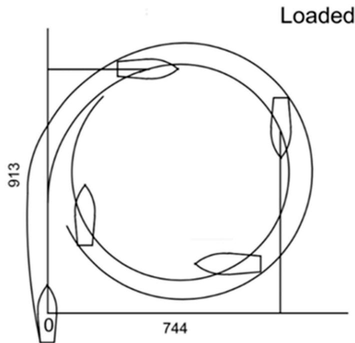
**Figure A1.** Turning circle at maximum rudder angle (sea trail).
