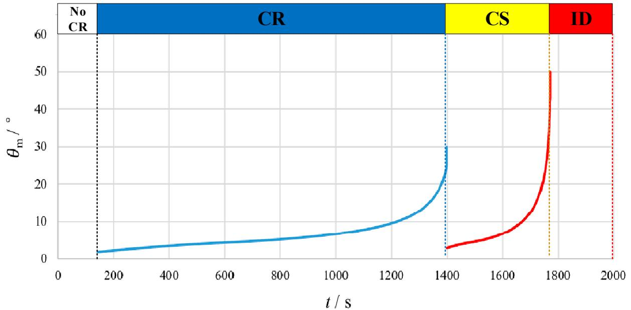
**Figure 14.** Minimum course-alteration angle for the stand-on vessel in an overtaking situation. The blue and red curves represent the minimum course-altering amplitude required to ensure that ship domain and collision domain are not invaded at different moments by the stand-on vessel in the risk of collision and close-quarter situation stages.
