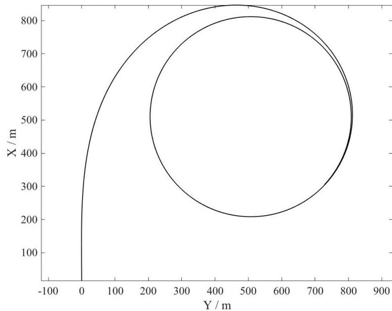
**Figure A2.** Turning circle at maximum rudder angle (digital MMG model).
