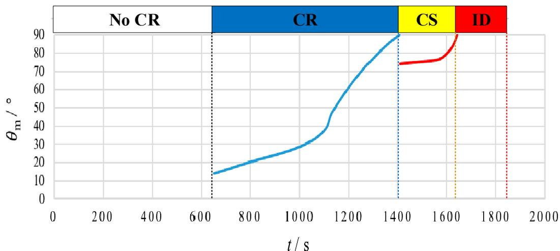
**Figure 10.** Minimum course-alteration angle for the stand-on vessel in a crossing situation. The blue and red curves represent the minimum course-altering amplitude required to ensure that ship domain and collision domain are not invaded at different moments by the stand-on vessel in the risk of collision and close-quarter situation stages.
