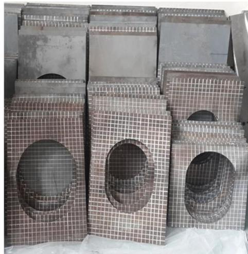
Figure 3. Specimens of the perforated plate after buckling experiment.
