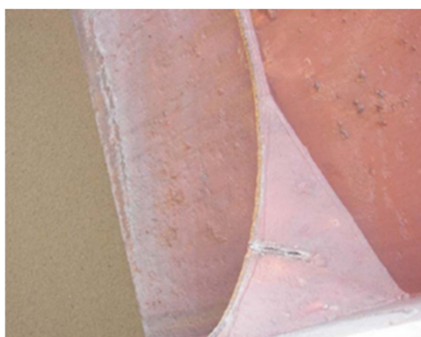
Figure 1. A fatigue crack in the hatch corner of a certain ship.
