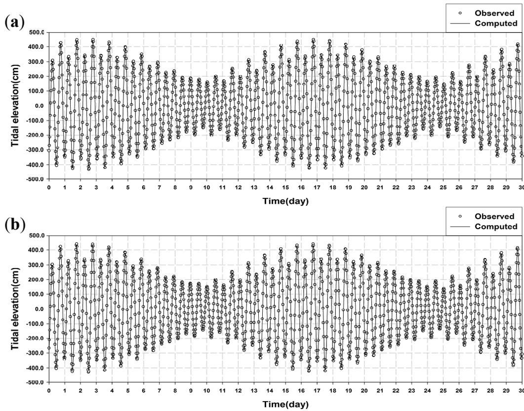
Figure 5. Computed tidal elevations using the EFDC model compared with the corresponding observed data at (a) T1 and (b) T2.
