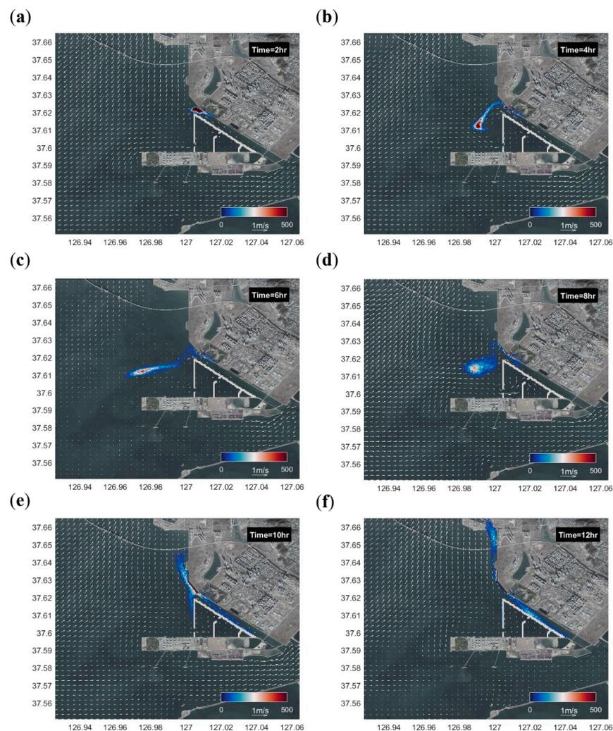
**Figure 16.** Temporal variation of the simulated oil concentration [ $\text{tonne}\cdot\text{km}^{-2}$ ] in (a) 2, (b) 4, (c) 6, (d) 8, (e) 10, and (f) 12 h after initiation in Scenario 3. Background vectors visualize tidal current fields.
