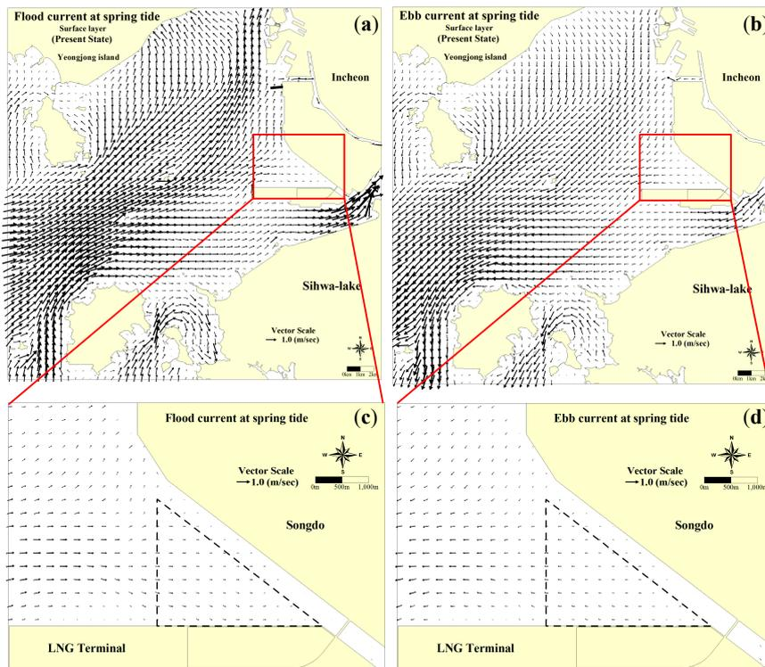
**Figure 11.** Current velocity fields in case 1 during the pre-construction phase without revetments installed. Current fields are shown in the enlarged views during (a) flood and (b) ebb and in the detailed domain near the LNG terminal construction site during (c) flood and (d) ebb.
