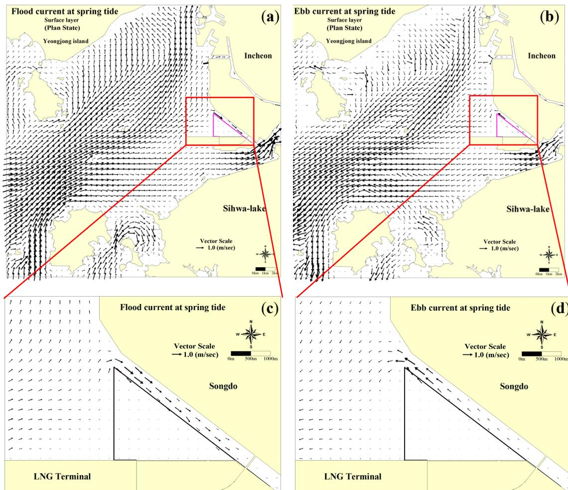
**Figure 13.** Current velocity fields in case 3, with both revetments and passages constructed. Current fields are shown in the enlarged views during (a) flood and (b) ebb and in the detailed domain near the LNG terminal construction site during (c) flood and (d) ebb.
