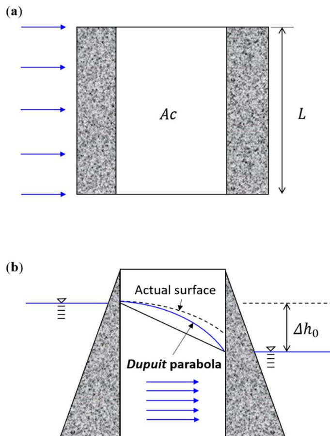
**Figure 9.** Schematic of the groundwater flow through permeable sea-dyke in (a) plan view and (b) side view.
