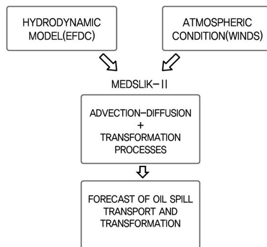
**Figure 1.** Schematic of the oil spill model (MEDSLIK-II) applied in the current study.
