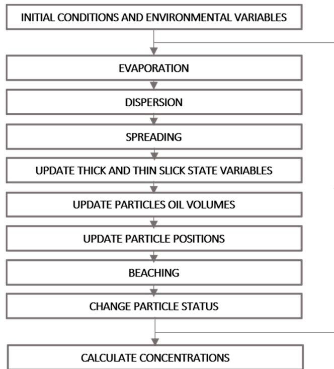
Figure 4. Computation flowchart in MEDSLIK-II.
