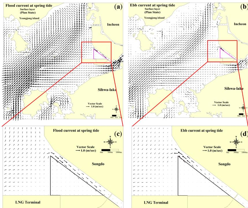
**Figure 12.** Current velocity fields in case 2 with only revetments were constructed without the seawater passages installed. Current fields are shown in the enlarged views during (a) flood and (b) ebb and in the detailed domain near the LNG terminal construction site during (c) flood and (d) ebb.
