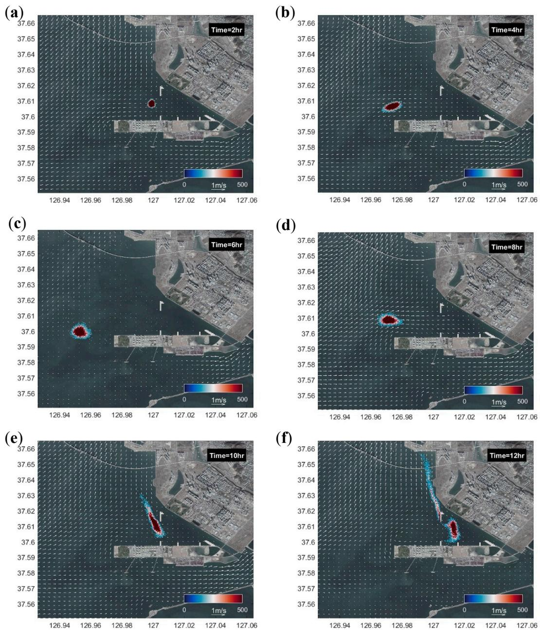
**Figure 14.** Temporal variation of the simulated oil concentration [tonne·km<sup>-2</sup>] in (a) 2, (b) 4, (c) 6, (d) 8, (e) 10, and (f) 12 h after initiation in Scenario 1. Background vectors visualize tidal current fields.
