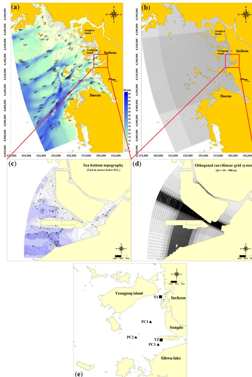
**Figure 2.** Bathymetry contours in meters in the (a) expanded and (c) detailed domain. The extent of a multilayered orthogonal curvilinear grid system in the (b) expanded and (d) detailed domain. (e) Enlarged view of target area. T1-T2 indicate the locations of the tidal elevation stations, and PC1-PC3 indicate the locations of the tidal current stations.
