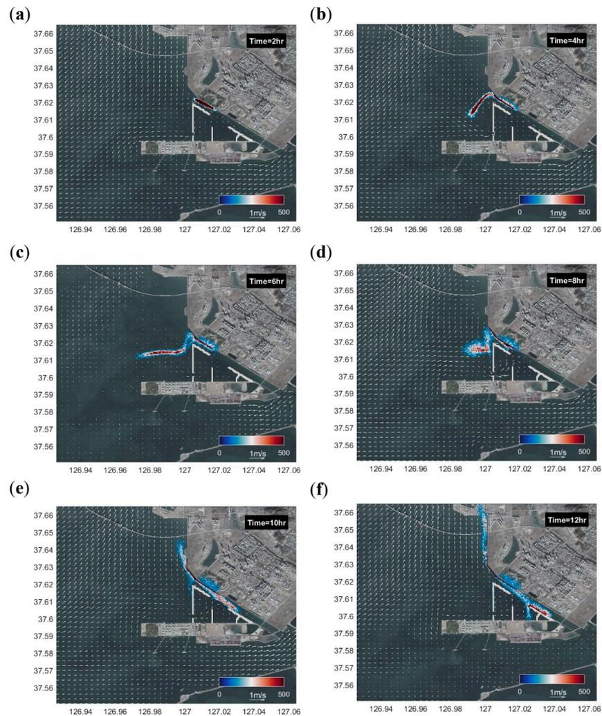
**Figure 15.** Temporal variation of the simulated oil concentration [tonne·km<sup>-2</sup>] in (a) 2, (b) 4, (c) 6, (d) 8, (e) 10, and (f) 12 h after initiation in Scenario 2. Background vectors visualize tidal current fields.
