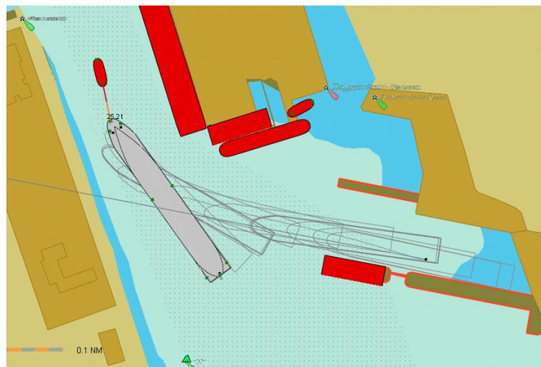
Figure 10. Ship’s trajectory on departure using one tug with bollard pull up to 500 kN (wind N—14 m/s).
