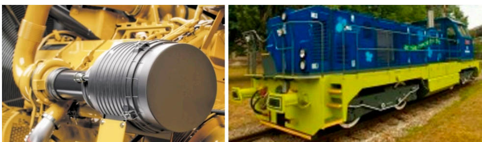
Figure 8. CNG engine and its application in an experimental rail vehicle.
