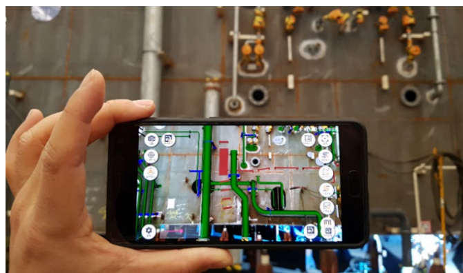
Figure 1. Installation inspection using proposed augmented reality (AR) system.
