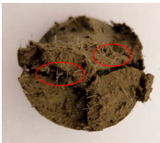
Figure 9. Sectional view of PCC after failure.
