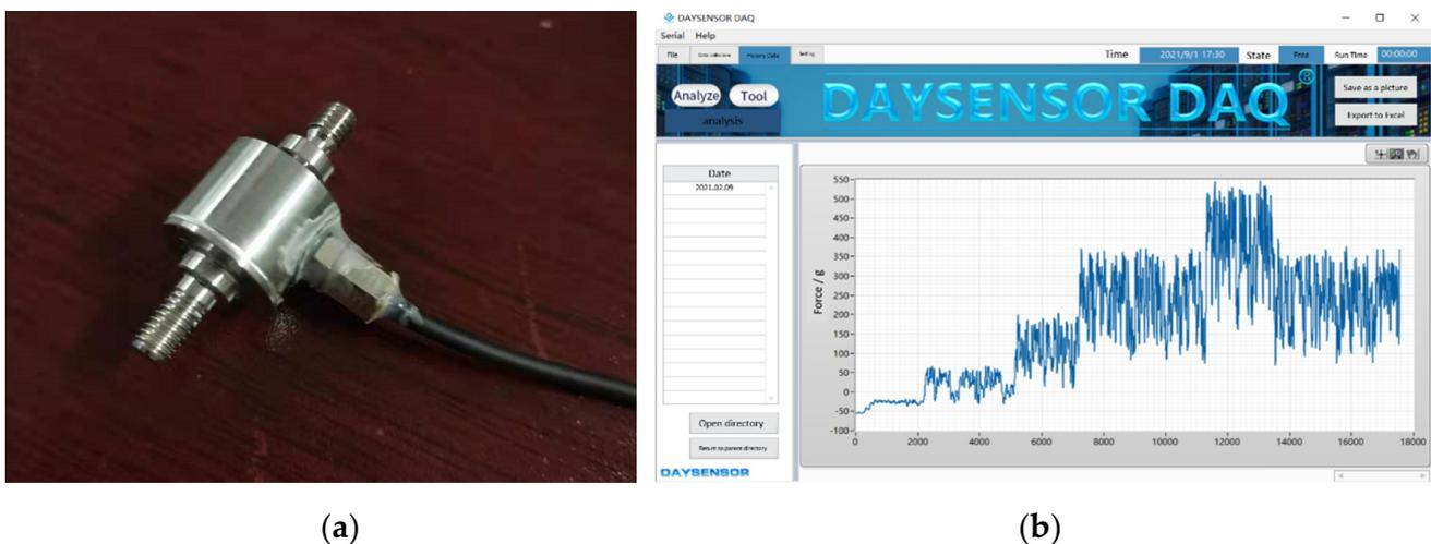
**Figure 6.** Data acquisition devices in detail, (a) DYMH-106D tension sensor; (b) Interface of DAY-SENSOR software.
