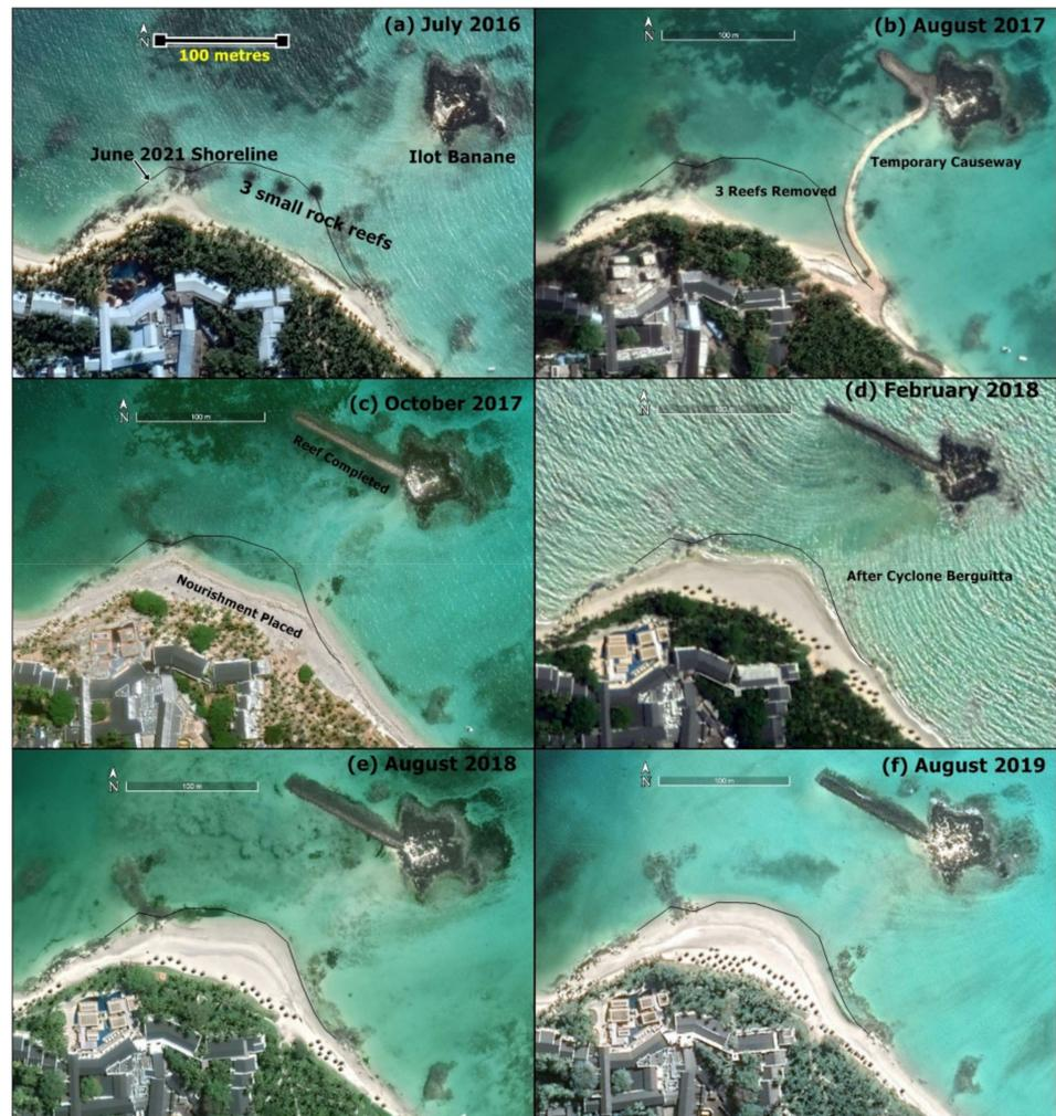
**Figure 5.** (a–f) Evolution of the salient at St Geran (Images from Google Earth). The black line shows the shoreline in June 2021. The February 2018 image (d) is after cyclone Berguitta. For scale, the reef is 95 m long. In (b), construction was undertaken in August–October 2017.
