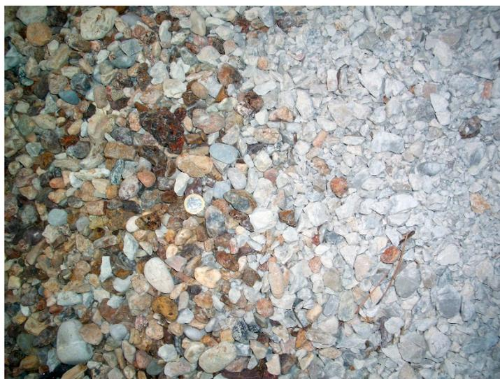
**Figure 5.** Fill materials used at Cavo: on the left side the iron rich mining waste, on the right side the new carbonate sandstone of the second nourishment. One euro coin for reference at the centre of the photo.
