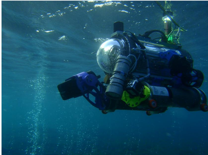
Figure 4. FeelHippo AUV during sea trials.
