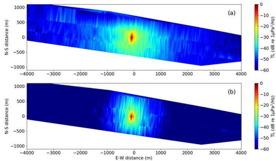
**Figure 4.** Spatial transmission loss for the two sonar systems on the CCGS Vector. Received sound pressure levels (SPL) relative to maximum SPL for the (a) 12 kHz and (b) 50 kHz sonars are shown.
