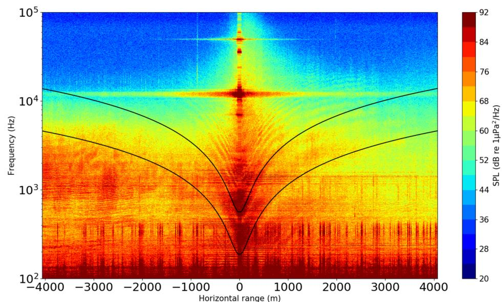
**Figure 3.** Spectrograms relative to the location of the PAM mooring for a transit of the CCGS Vector at a constant speed at 1500 RPM. The first two Lloyd's mirror effect peaks are highlighted with black lines. The vessel is travelling from left to right.
