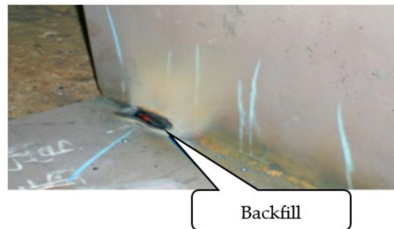
**Figure 19.** Bead backfill.
