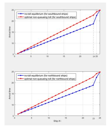
**Figure 3.** Numerical results of arrival time adjustment for southbound (SB) and northbound (NB) ships from the no-toll to the tolled case.
