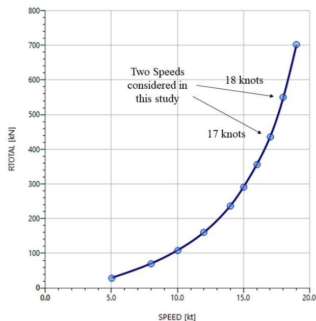
**Figure 2.** Total resistance of the container ship at different speeds.
