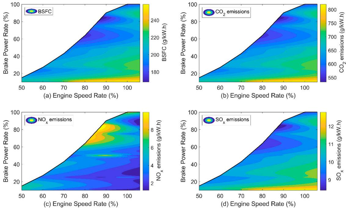
**Figure 3.** Load diagram of marine diesel engine. (a) BSFC (b) CO<sub>2</sub> emissions (c) NO<sub>x</sub> emissions (d) SO<sub>x</sub> emissions [38,46].
