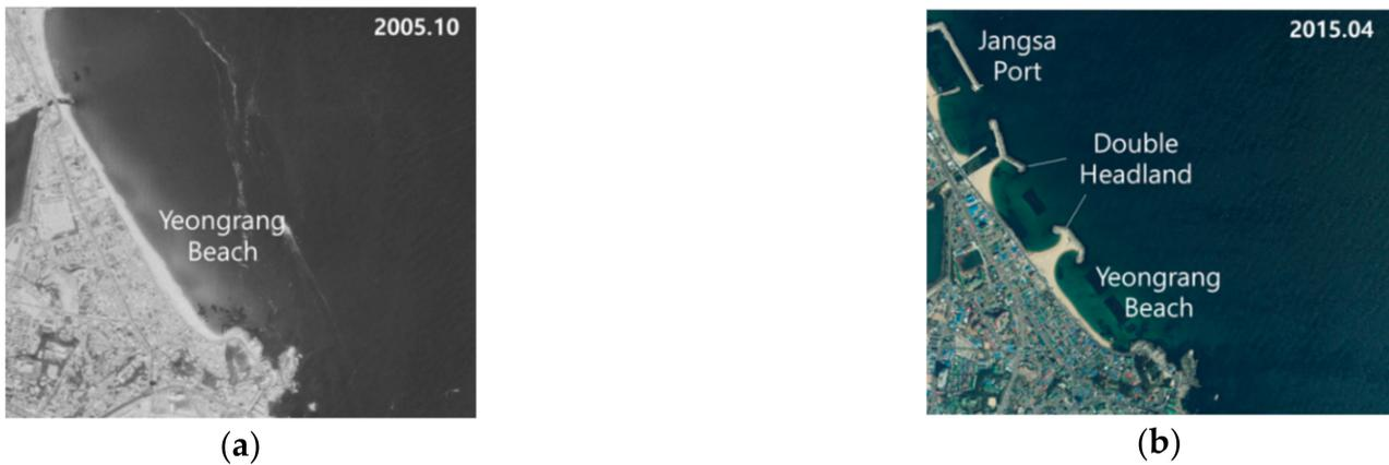
**Figure 13.** Yeongrang beach before and after construction of double headland: (a) October 2005 (image from NGII); (b) April 2015 (image from NGII).
