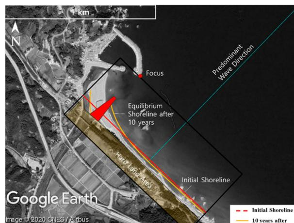
**Figure 17.** Results of model simulation to reduce erosion of Wonpyeong beach by repositioning groin (image from Google Earth as at October 2012).
