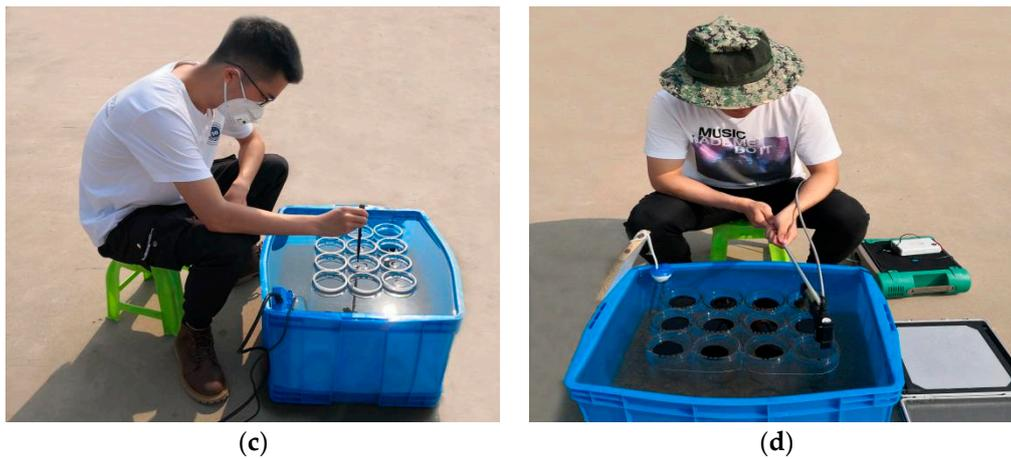
**Figure 2.** Photos of the field experiment. (a) Experimental container after adding oil. (b) Weighing crude oil mass. (c) Adding crude oil to the container. (d) Oil film spectral data measurement.
