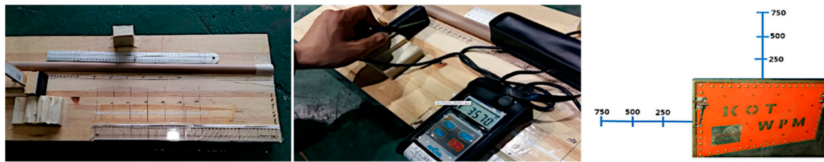
Figure 10. Magnetic field test. From left to right: fixing the magnet's position; checking its magnetic field; checking the magnetic field of the device.
