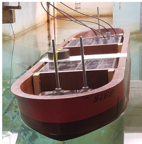
Figure 9. Model during Incline Test.
