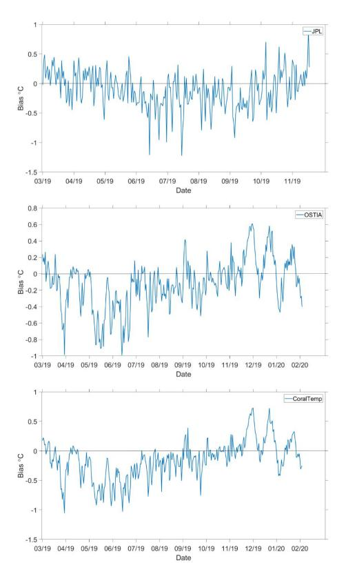
**Figure 6.** Time series of the bias (satellite—in situ) temperatures from 1 March 2019–1 March 2020 for San Cristobal.
