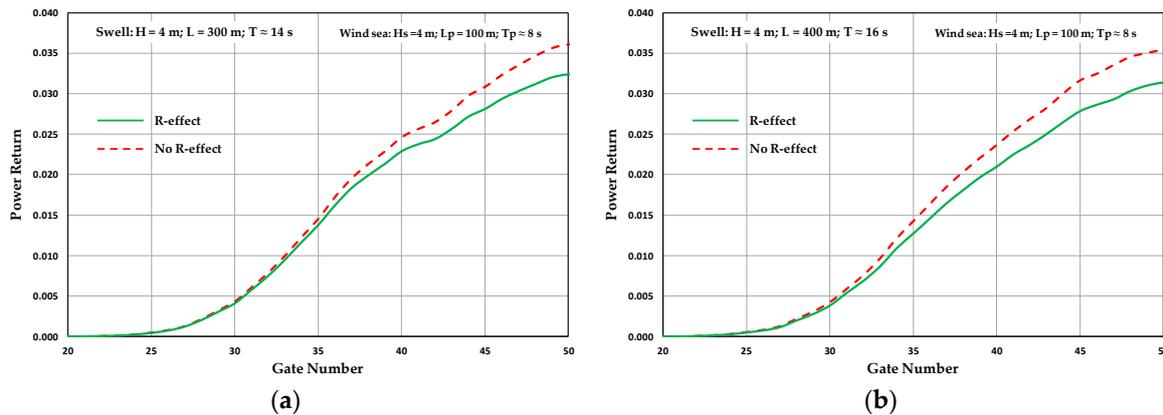
**Figure 10.** Comparison between averaged 20 Hz WF with (green line), and without (dashed red line), R-effect for swell superimposed to a wind sea: (a) JONSWAP significant wave height  $H_s = 4$  m, peak wave period  $T_p = 8$  s; swell wave height  $H = 4$  m, period  $T = 14$  s; (b) JONSWAP significant wave height  $H_s = 4$  m, peak wave period  $T_p = 8$  s; swell wave height  $H = 4$  m, period  $T = 16$  s.
