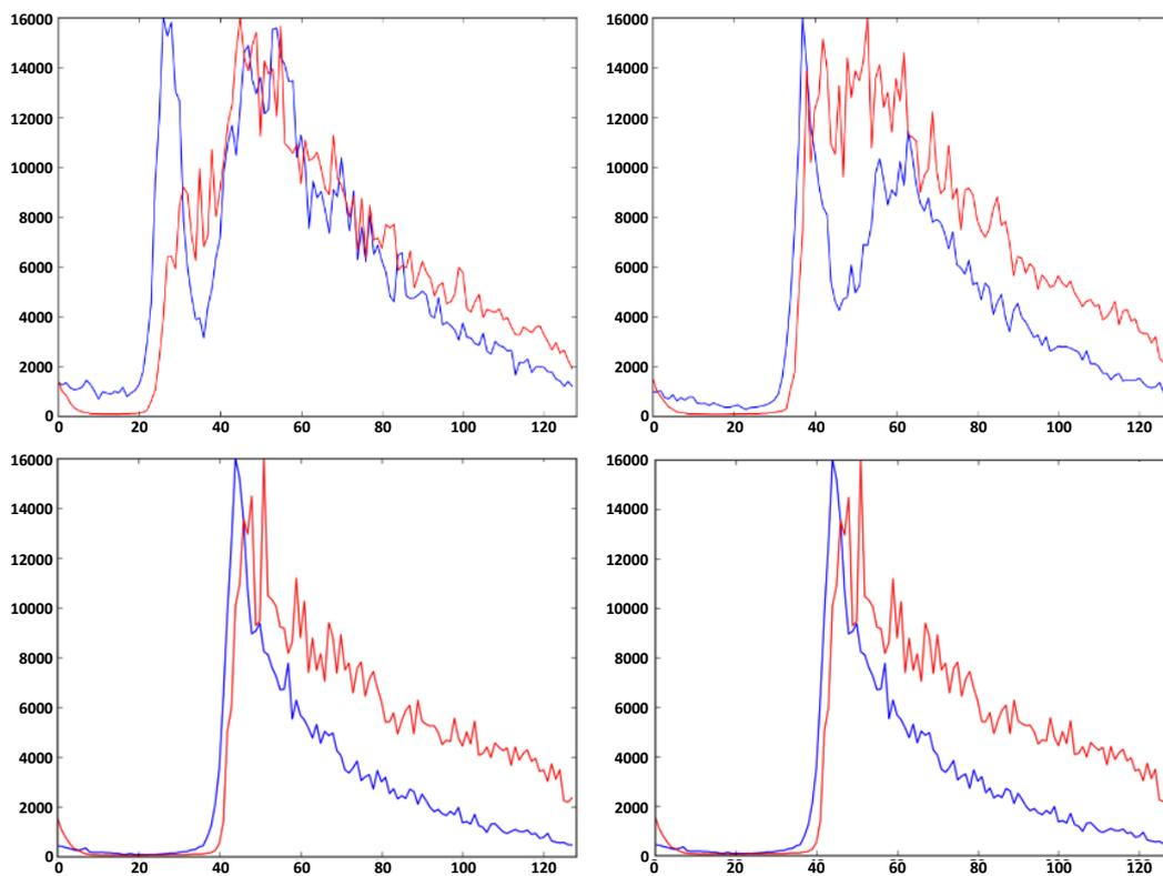
**Figure 1.** Experimental waveforms both in delay Doppler altimeter (DDA) mode (blue line) and conventional altimetry mode (red line) for various swell events detected by CryoSat-2 altimeter (track 681, cycle 030) as reported in [11].
