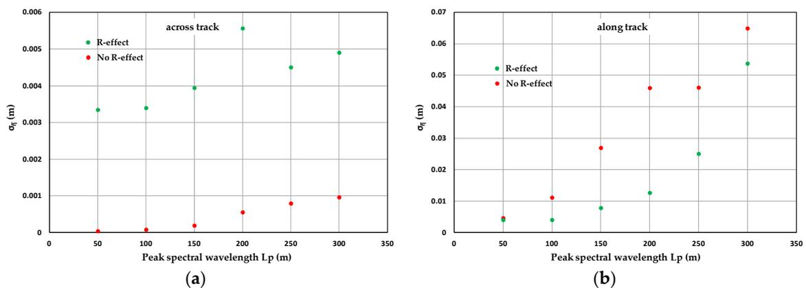
**Figure 12.** Standard deviation values  $\sigma_{\bar{\eta}}$  as a function of peak spectral wavelength  $L_p$  by considering (green diamonds), and by neglecting (red circles), R-effect: (a) main wave direction across satellite track; (b) main wave direction along satellite track.
