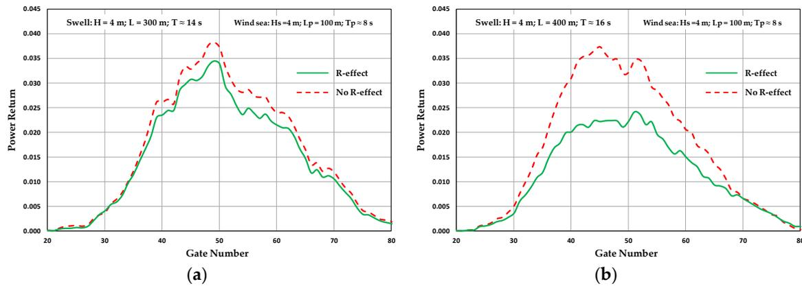
**Figure 9.** Simulated single waveforms with (solid green line), and without (dashed red line), R-effect for swell superimposed to a wind sea: (a) JONSWAP significant wave height  $H_s = 4$  m, peak wave period  $T_p = 8$  s; swell wave height  $H = 4$  m, period  $T = 14$  s; (b) JONSWAP significant wave height  $H_s = 4$  m, peak wave period  $T_p = 8$  s; swell wave height  $H = 4$  m, period  $T = 16$  s.
