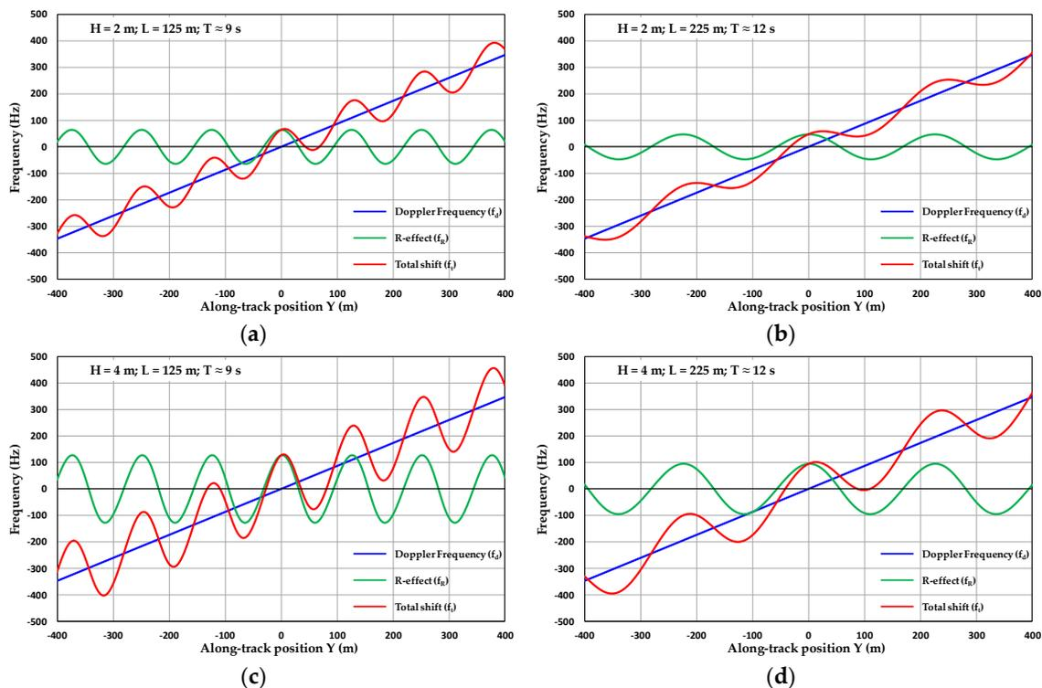
**Figure 5.** Along-track Doppler frequency shift values for different sinusoidal waves: (a) wave height  $H = 2$  m, wavelength  $L = 125$  m, wave period  $T \approx 9$  s; (b)  $H = 2$  m,  $L = 225$  m,  $T \approx 12$  s; (c)  $H = 4$  m,  $L = 125$  m,  $T \approx 9$  s; (d)  $H = 2$  m,  $L = 225$  m,  $T \approx 12$  s.
