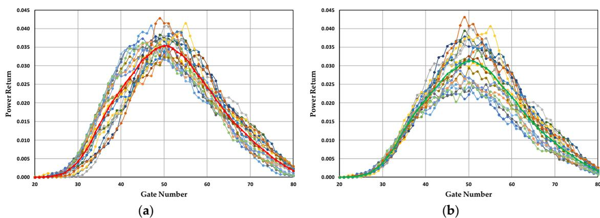
**Figure 8.** Simulated waveforms on a 20 Hz sample for sinusoidal wave train (wave height  $H = 4$  m,  $T = 16$  s) superimposed to a JONSWAP sea (significant wave height  $H_s = 4$  m; peak period  $T_p = 8$  s): (a) without R-effect (red curve represents the average value); (b) with R-effect (green curve represents the average value).
