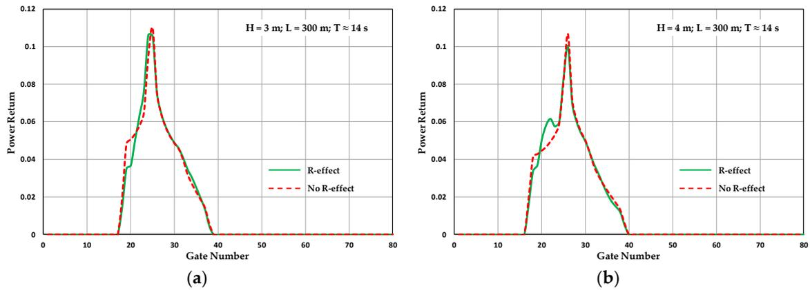
**Figure 6.** Simulated waveform with (solid green line), and without (dashed red line), R-effect for two different single sine wave trains: (a) wave height  $H = 3$  m, wavelength  $L = 300$  m, wave period  $T \approx 14$  s; (b)  $H = 4$  m,  $L = 300$  m,  $T \approx 14$  s.
