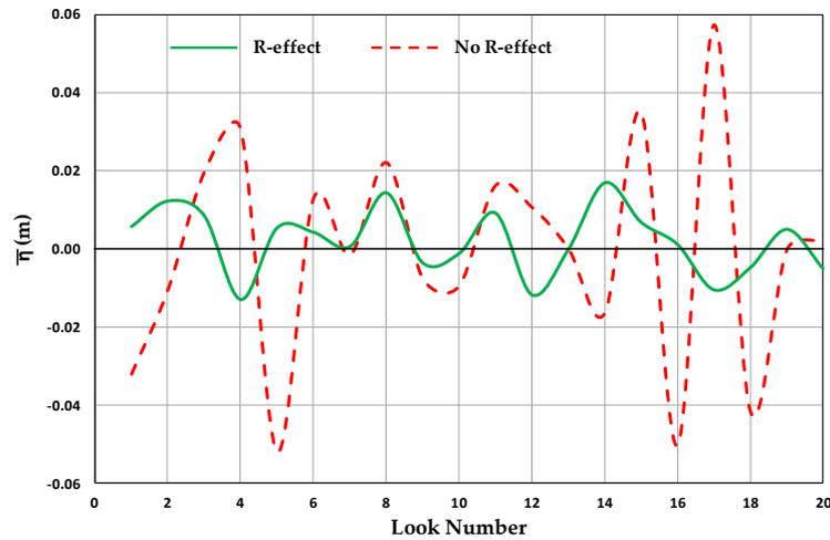
**Figure 11.** Sea surface height average values  $\bar{\eta}$  by taking in account (solid green line), and by neglecting (dashed red line), the R-effect.
