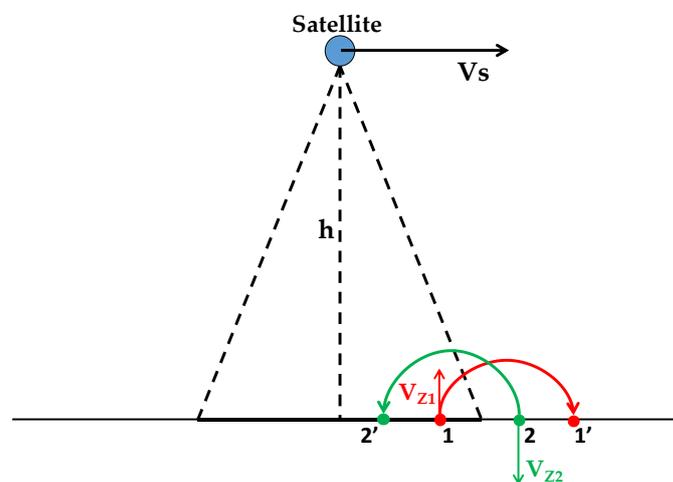
Figure 4. Effect of particle vertical velocity on the apparent position of an elementary surface area. The red point, positioned in 1, has a positive vertical velocity component  $V_{Z1}$ , which adds to its  $V_c$ ; it therefore appears to be farther (position 1') from the nadir; the green point, positioned in 2, has a negative  $V_{Z2}$ ; it therefore looks closer (position 2').
