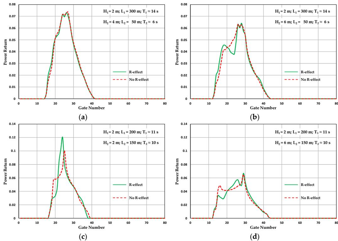
**Figure 7.** Simulated waveform with (solid green line), and without (dashed red line), R-effect when a longer sinusoidal wave train (wave height  $H$ , wavelength  $L_1$ ) is superimposed to a shorter one (wave height  $H_2$  and wavelength  $L_2$ ): (a)  $H_2 = 4$  m,  $L_2 = 50$  m; (b)  $H_2 = 6$  m,  $L_2 = 50$  m. (c)  $H_2 = 2$  m,  $L_2 = 150$  m; (d)  $H_2 = 6$  m,  $L_2 = 150$  m.
