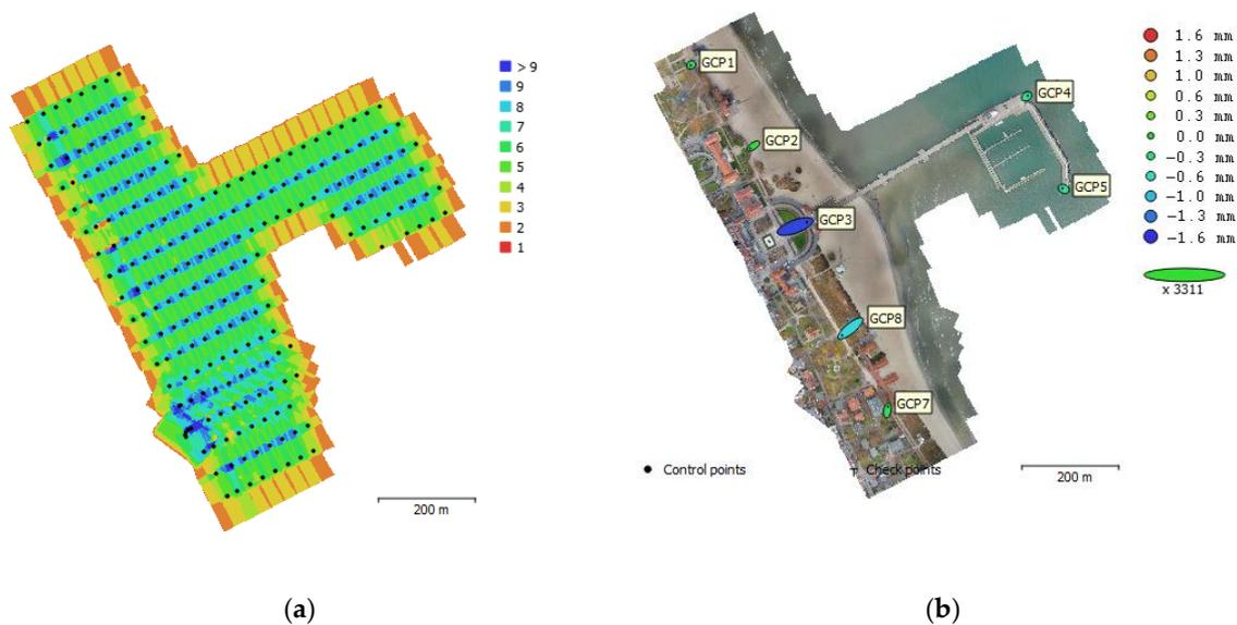
**Figure 3.** The location of the camera and the overlap (the number of images that present a particular surface is marked with appropriate colors) (a) and the distribution of control points with the position error indicated (the horizontal position error by the ellipse shape and the vertical position error is presented by the ellipse color) (b).
