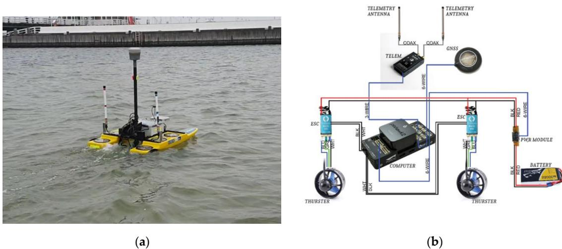
**Figure 2.** Unmanned Surface Vehicle (USV) with measuring equipment mounted to it (a) and a schematic diagram of the main components of the USV after the modernization of the control system from remote to automatic mode (b) [57].
