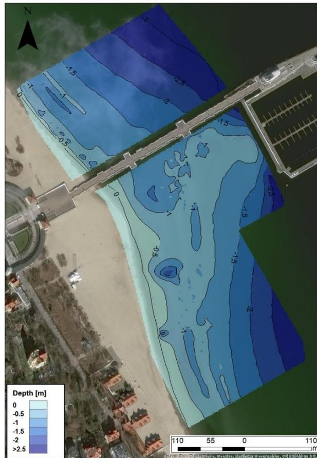
**Figure 6.** A bathymetric chart of the waterbody adjacent to the Sopot pier, developed based on hydrographic and photogrammetric measurements carried out in November 2019.
