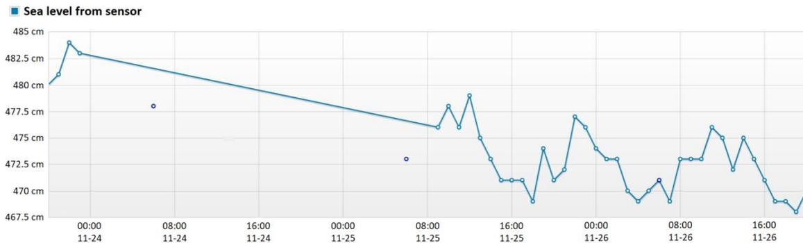
**Figure 5.** A diagram of sea level variability observed on a tide gauge in Gdynia according to the Institute of Meteorology and Water Management—National Research Institute (IMGW—PIB) weather service.
